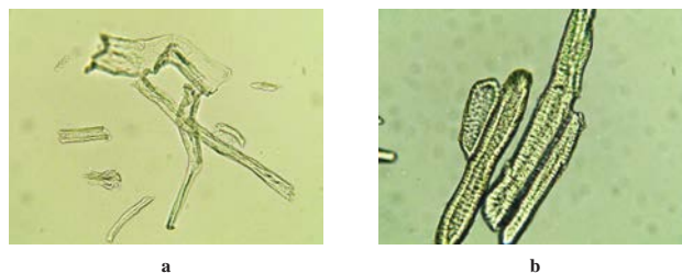
Fig. 1. Fibrous filler particles derived from: corn stalks (a); coconut shells (b)
